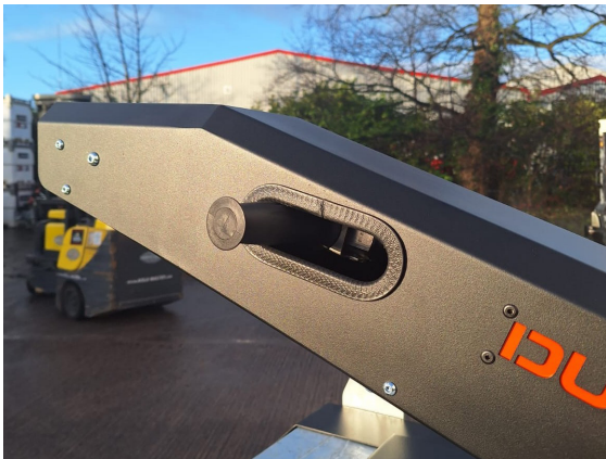
Lever in raised position for Jet
